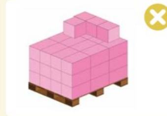
Pyramid stacking will affect the stability during the transit, and increase the risk of damages and make it dangerous to unload.
