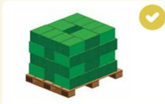
Interlock stacking by various carton size.
